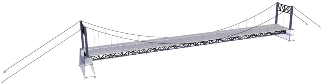
Figure 16: Global finite element model of the Ölfusá Suspension bridge.
